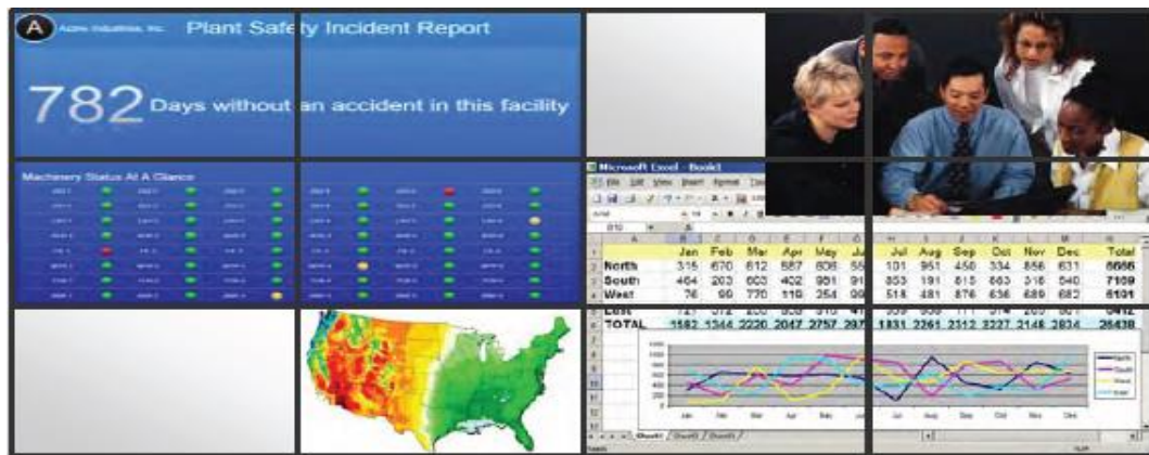
4x3 NEC Display Video Wall – 12x Slot-in PC connected via LAN
